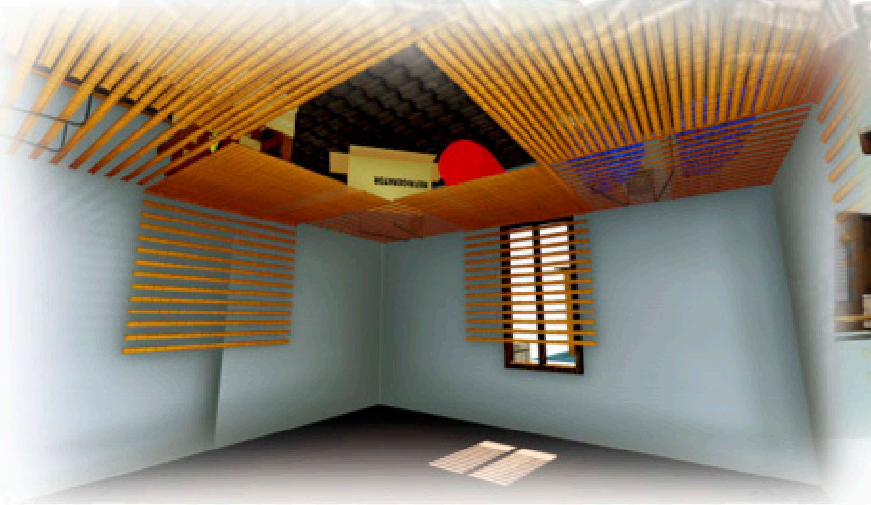
APART FROM TEMPORARY STORING OF HOUSEHOLD STUFF, THE DOUBLE LAYERED MIDDLE SEGMENTS MIGHT BE USED FOR PARTIAL SHADING OF DOORS AND WINDOWS, ALSO INCREASING SECURITY IN DWELLINGS LIKE SLUMS.
